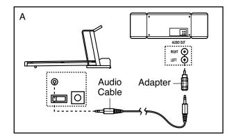
B. Plug one end of the audio cable into the jack on the front of the treadmill near the power cord. Plug the other end of the cable into the LINE OUT jack on your stereo.
